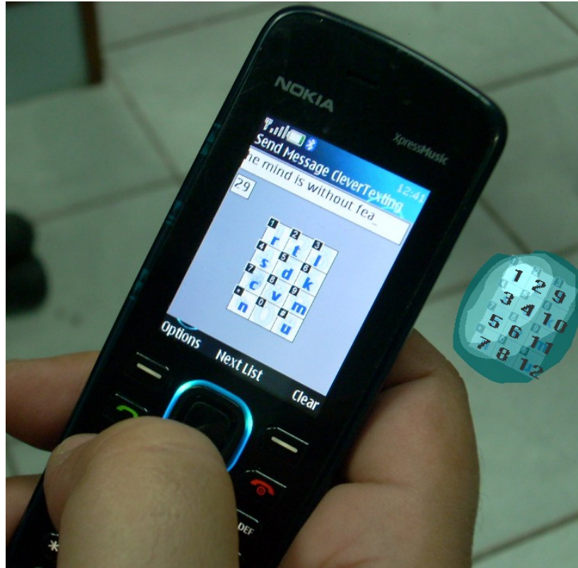
CleverTexting anticipating characters most likely to be entered next and placing them on positions most comfortable for your texting thumb from which you can type using single key tap. See the Ergonomic ranks and contours shown on the right.
