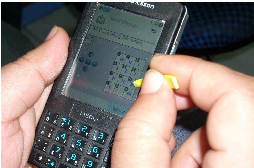
CleverTexting being used on a Touchscreen phone in Nearest Key Mode.
